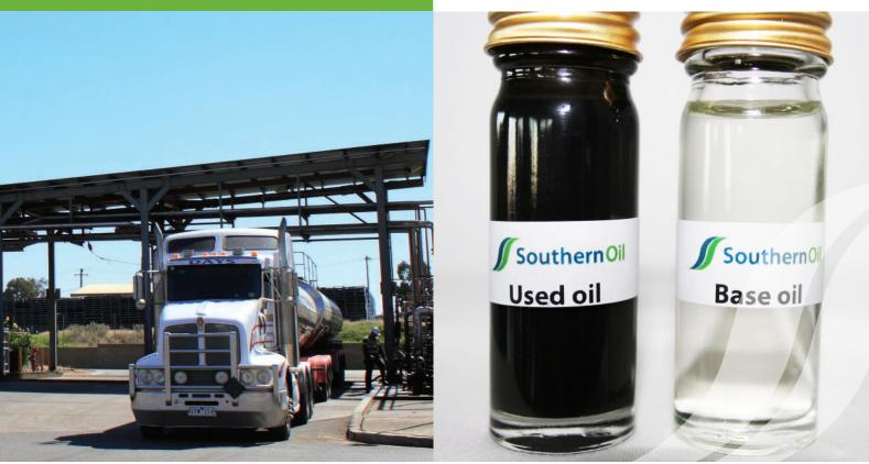
(Left) unloading waste lube oil at Wagga Wagga; (right) used lube oil comes in and is re-refined into base oil
